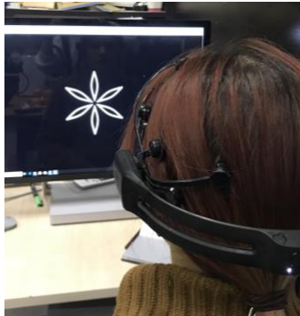
Figure 1: The subject is taking the experiments with a head-mounted EMOTIV equipment and the tests in the browser. Every test takes about 1 hour, including the self-assessment manikin (SAM) and the EEG data by EMOTIV EPOC+ for the same content. These 10 tests include the number, morphology, hue, saturation, brightness, scale, rotation and motion speed to test their effects of the petals on people.
